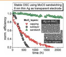
A stable semitransparent thin silver top contact for organic solar cells is fabricated by sandwiching it between thermally evaporated MoO<sub>3</sub> layers. By using a MoO<sub>3</sub> interlayer, the morphology of the Ag electrode is improved, leading to better charge collection. The sandwich increases the electrode transmittance, photocurrent generation, and lifetime. With this, more efficient solar cells with lifetimes of 4500 h are achieved.
