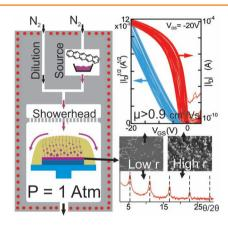
The effect of carrier gas pressure on the growth of pentacene by organic vapor phase deposition is explored. At high pressures (>100 mbar), gas phase nucleation is observed, which results in rough layers. An optimized process window is defined to grow smooth pentacene thin films at atmospheric pressure. State-of-the-art transistors and circuits based on these films are demonstrated.
