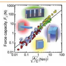
Design criteria for bio-inspired adhesives under shear loading is presented. Force capacity predictions of common geometric control parameters such as thickness, aspect ratio, and contact area are experimentally confirmed. This understanding is extended to over 25 simple and complex adhesive patterns. The force capacity of the various attachment features is described with a simple scaling parameter.
