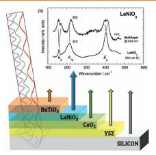
The integration of functional oxides on silicon requires the use of complex heterostructures where the structure and properties strongly depend on the strain state. A Raman study of a multilayer BaTiO<sub>3</sub>/LaNiO<sub>3</sub>/CeO<sub>2</sub>/YSZ thin-film structure on silicon is reported, demonstrating that wavelength-dependent Raman scattering is well adapted for the investigation of strain and structural changes in complex heterostructures or even nanocomposites.
