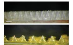
Microneedle arrays prepared from crosslinked polymers, which contain no drug themselves, are described. They rapidly take up skin interstitial fluid upon skin insertion to form continuous, unblockable, hydrogel conduits from attached patch-type drug reservoirs to the dermal microcirculation. This technology has the potential to further enhance the capabilities of microneedle strategies for transdermal drug delivery, while bypassing current difficulties.
